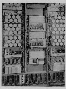
Proper formation of the image is achieved through the synchronizing signal-generator. Its intricacies are revealed in this view
