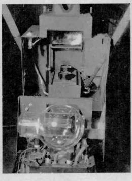
Inside the camera, center, is the iconoscope, or "television eye." The plate inside tube changes light to electrical waves
